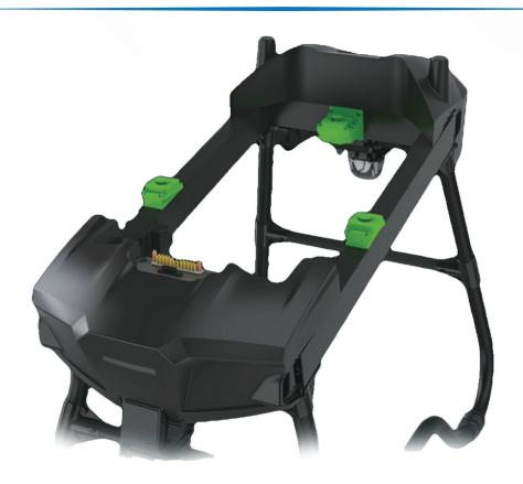
Weight sensor real-time remaining pesticide monitoring
